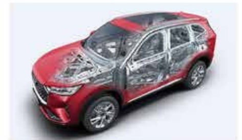
71.61% high-strength steel body
