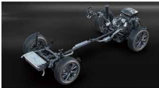
Front Macpherson rear multi-link independent suspension + AWD
