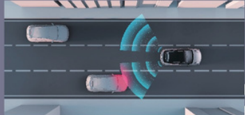
BSD (Blind Spot Detection) system
