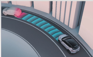
ACC (Adaptive Cruise Control) system
